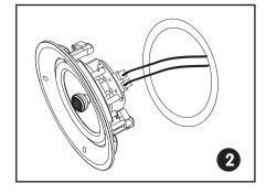
Connect the speaker wires to the speaker.
