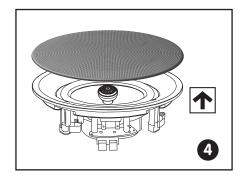
Press the cover according to the direction of the picture with the speaker assembly.
