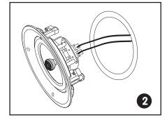
Connect the speaker wires to the speaker.
