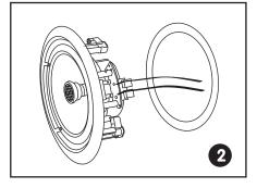
Connect the speaker wires to the speaker.
